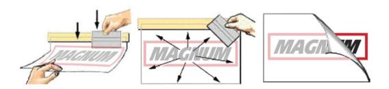
While still holding the PRE-MASKed graphic away from the window surface, use a squeegee (supplied) or any plastic straight edge to help in application. Start from the side with the tape and gently work away from the tape and squeegee out all water and soap.
